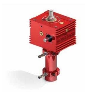
Limit switches can be mounted on the screw jacks cover pipe to signal stroke positions such as end of travel. The switch is triggered by a cam or target disc on the end of the lead screw.
